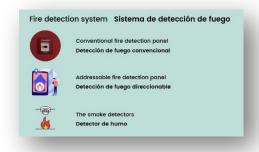
Also related to security, an electronic technician can install a fire detection system Sistema de detección de fuego and its peripheral devices Dispositivos periféricos including either a conventional Convencional or an addressable fire detection panel Direccionable. The peripherals include either simple or addressable smoke detectors and activation modules for electrovalves. The smoke detectors Detector de humo can be either photoelectric or beam.
