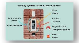
Security at home is an important issue nowadays. An electronic technician can provide reliable solutions to ensure the buildings' security. They can install a security system Sistema de seguridad and all the peripheral devices including the central control panel Panel de control with embedded siren Sirena and keypad Teclado, the magnetic traps Trampa magnética and the outdoors siren or beacon Baliza.
