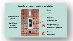
Security at home is an important issue nowadays. An electronic technician can provide reliable solutions to ensure the buildings' security. They can install a security system systima asfaleias and all the peripheral devices including the central control panel kentrikos pinakas elenchou with embedded siren sirina and keypad pliktrologio, the magnetic traps magnitiki pagida and the outdoors siren or beacon farosirina.
