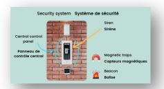
Security at home is an important issue nowadays. An electronic technician can provide reliable solutions to ensure the buildings' security. They can install a security system Système de sécurité and all the peripheral devices including the central control panel Panneau de contrôle central with embedded siren Sirène and keypad, the magnetic traps Capteurs magnétiques and the outdoors siren or beacon Balise.
