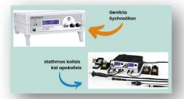
Other instruments you will use are Function Generators Genitria Sychnotiton and soldering and desoldering stations stathmos kolisis kai apokolisis.
