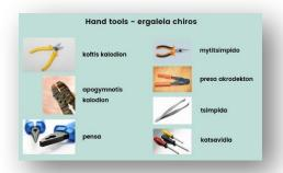
The most common tools for an electronics technician are the hand tools ergaleia chiros. These tools are wire cutters koftis kalodion, wire strippers apogymnotis kalodion, normal pliers pensa and long nose pliers mytitsimpido, plug crimping pliers presa akrodekton, tweezers tsimpida, and screwdrivers for electronics katsavidia.
