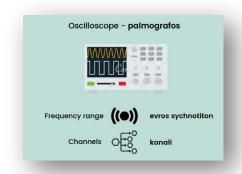
The oscilloscope palmografos is a state of the art instrument for an electronics laboratory. You will either use an analogue or a digital one. It is important to know which frequency range evros sychnotiton you want to work with. How many channels kanali you need for measuring and the accessoiries that will be useful to carry out the tasks.
