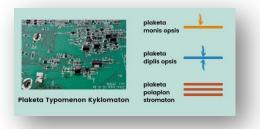
The most common electronic component you have to work with as an electronic technician is the PCBs, the Printed Circuit Boards Plaketa Typomenon Kyklomaton. They support and connect electronic components using conductive tracks. PCBs could be single-sided plaketa monis opsis, double-sided plaketa diplis opsis or multi-layer plaketa polaplon stromaton.
