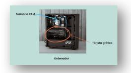
which stores snapshot data submitted to the processor, the graphics card, Tarjeta gráfica which allows the display graphics on a PC screen.
