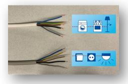
One of the cables has single-wire rigid copper cores. The other has finely stranded flexible copper cores. starre Kupfer-Adern flexible Kupfer-Adern The cores of both cables have the same cross section: Querschnitt. They can therefore be loaded with the same current. Cables with rigid copper cores are used for fixed installation, for example in the wall.
