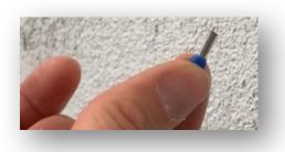
Wire end sleeves must be pressed onto flexible copper wires with crimping pliers: Aderendhülse. This ensures a permanent connenction!
