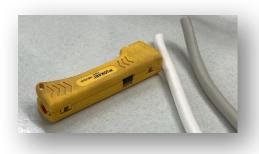
Let's take a closer look at two sheathed cables for electrical power supply. We remove the sheath insulation with a stripper Entmantler without damaging the cores.
