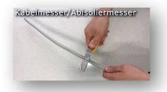
For longer pieces, use a cable knife/stripping knife: Kabelmesser.
