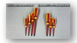
Screwdrivers are needed in different sizes. Slot screwdriver - Schlitzschraubendreher Phillips screwdriver – Kreuzschlitzschraubendreher They must be insulated up to 1000 V for safety.
