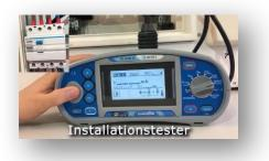
The safety of an electrical installation is measured with an installation tester: Installationstester. For example, the correct function of a residual current circuit breaker.
