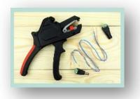
The insulation of the individual wires is removed with a wire stripper: Apogymnotis kalodion.
