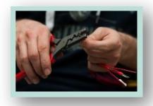
Crimping pliers are used to press sleeves or cable lugs onto finestranded wires: Presa akrodekton.
