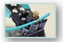
Remove the sheath insulation of the cable without damaging the insulation of the cores.
